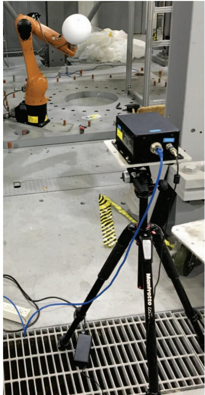
**Figure 5. The OS is mounted on the KUKA robotic arm and driven in a straight line trajectory towards the LiDAR**
